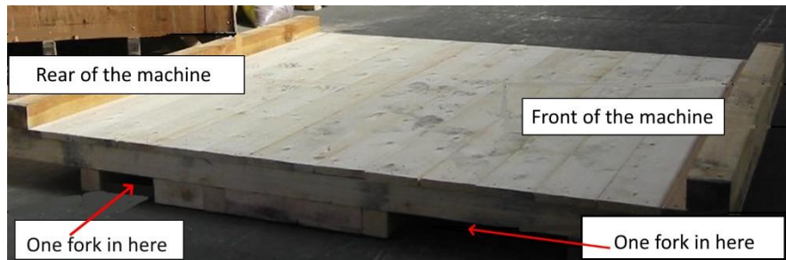
Figure 4 - Pallet forklift zones
